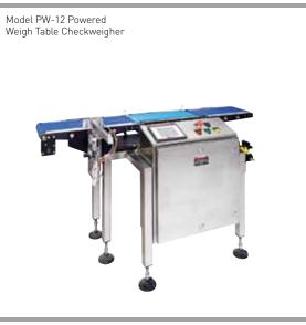
Data Output: RS-232, RS-422, Ethernet, other Feedback: Contact closure, digital, dual/single head filler, custom
