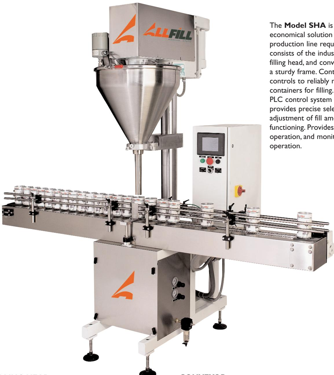
The **Model SHA** is a complete, economical solution to your filling production line requirements. It consists of the industry-proven All-Fill filling head, and conveyor mounted on a sturdy frame. Container indexing controls to reliably move and position containers for filling. Allen Bradley PLC control system with touchscreen provides precise selection and adjustment of fill amounts and machine functioning. Provides easy setup, operation, and monitoring of the filling operation.
